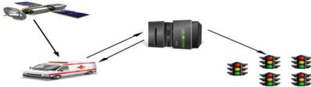
Fig. 4 Communication between ambulance vehicle, Satellites, web server and traffic LED
